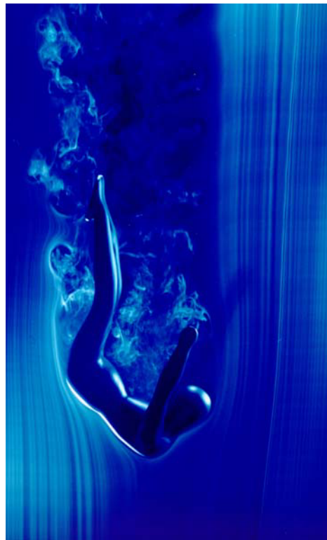
Fig. 1. Smoke wire flow visualization in the windtunnel
